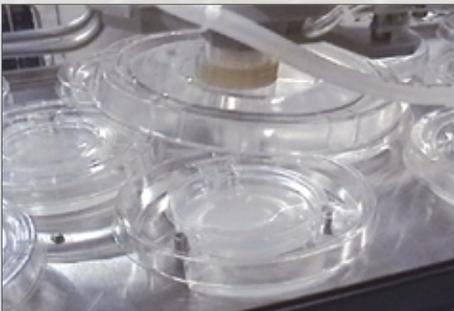
When the trays are returned to the system after undergoing ancillary operations, the robot moves the end effector to again remove the petri dish cover and this time aspirates the product from the well and dispenses another dose of product into two wells. The product tray is tilted to facilitate required aspiration and minimize residual product. These processes continue until the product has completed dispensing and aspirating the required cycles.
