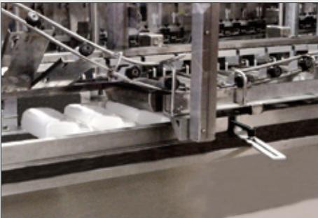
Filled and capped bottles are delivered to the system at 260 bottles/minute via a standard conveyor equipped with tabletop chain where they enter a timing screw. The timing screw releases the bottles in groups of three or four in synchronization with corresponding platens.
