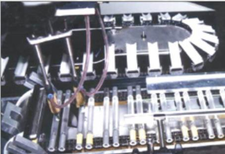
A 2-axes pick and place receives a signal from a conveyor sensor that the next row of vials from the oven conveyor and places them down into a pair of round belt conveyors whose direction of travel is perpendicular that of the oven conveyor.
