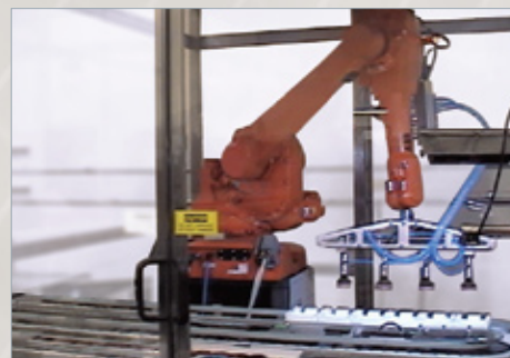
8. Robotic puck unloader
