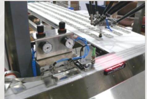
3. Vision acquisition – picking and placing
