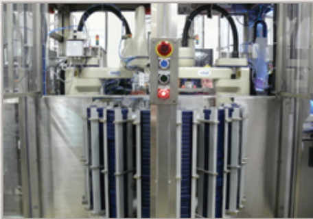
1. Rotary indexing product magazine
