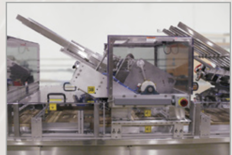
Thiele placers with Farason servo drives
